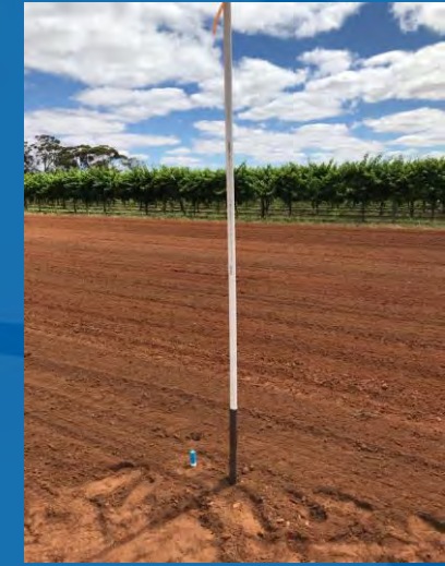
Soil moisture probes
