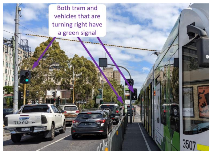
Figure 20: Parallel green phase for tram and vehicles at Lygon St / Princes St (Source: Lexus Australia)
